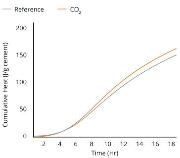
$CO_2$  injection improves cement hydration, allowing for up to 5% reduction in cement content without compromising performance. By optimizing  $CO_2$  dosage, both technical efficiency and economic viability are enhanced, achieving equal or superior concrete performance with less cement. This leads to cost savings and a reduced environmental footprint.
