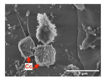
This  $CO_2$  mineralization reaction occurs while the concrete is still fresh, and differs from atmospheric carbonation, where  $CO_2$  predominantly reacts with CH. The formation of calcium carbonate minerals positively influences the cement hydration process, contributing to overall performance improvements and without affecting pore water pH.
